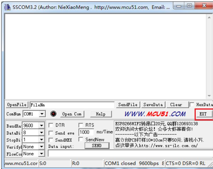
(3) Baud rate should be 9600. Tick HEX and HexData so that the command can be received by the Serial MP3 Player and you can see the feedback information in the blank of the window. Before sending commands, you should select the [ComNum] and click [Open Com].
