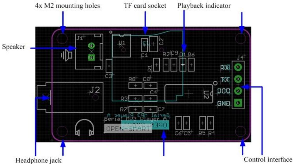
**Control interface:** It is UART TTL interface. A total of four pins (GND, VCC, TX, RX), GND to ground, VCC is the power supply, TX is the TX pin of the MP3 chip, RX is the RX pin of the MP3 chip.
